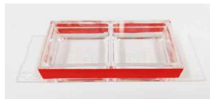
Figure 1. When taking images through confocal microscopy, the image chamber must be seal by label tape.
