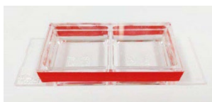
Figure 2. When taking images through confocal microscopy, the image chamber must be seal by label tape.
